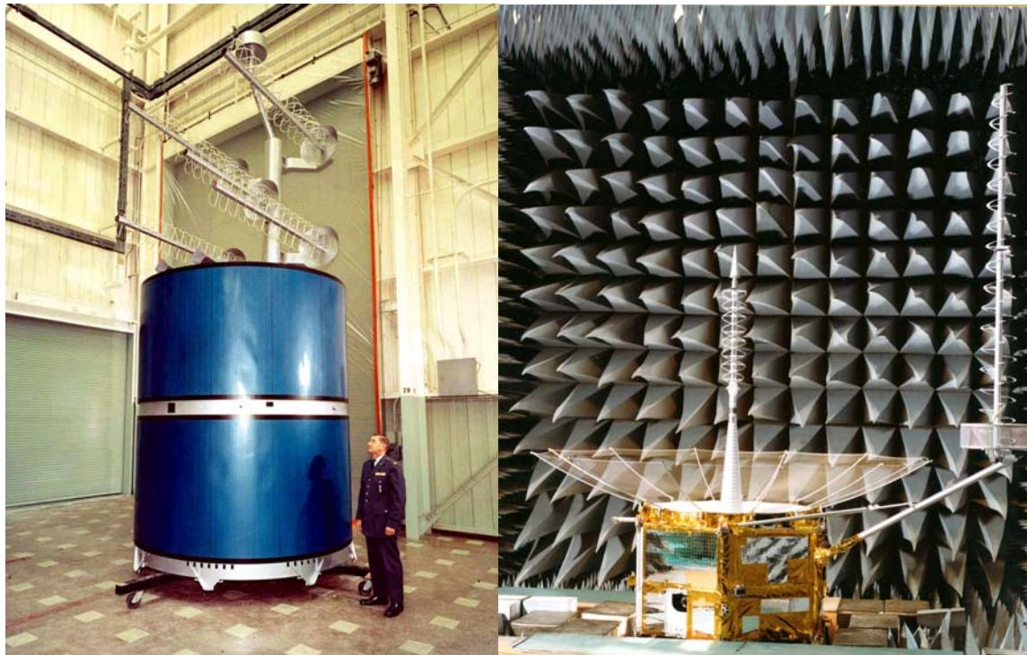
*Left: SAMSO's TACSAT program director poses with TACSAT I in the testing facilities of the prime contractor, Hughes Aircraft Company, about 1969. SAMSO launched TACSAT using a Titan IIIC on 9 February 1969, and it operated successfully for 46 months. Right: A FLTSATCOM satellite undergoes testing in an anechoic test chamber.*
