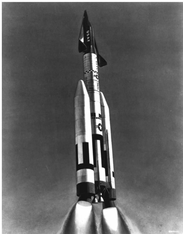
*Left: An artist's concept of the Dyna-Soar system depicts the Titan IIIC launch vehicle developed by AFBMD and the manned, aerodynamic vehicle developed by Wright Air Development Center. The program was canceled in 1963 before flying any hardware, but AFBMD and its successors proceeded to develop the Titan IIIC into one of the most important launch vehicles in the Air Force inventory*
