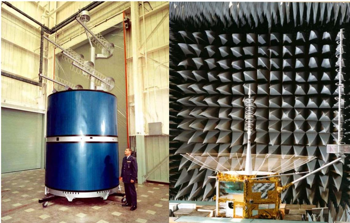
*Left: SAMSOC's TACSAT program director poses with TACSAT I in the testing facilities of the prime contractor, Hughes Aircraft Company, about 1969. SAMSOC launched TACSAT using a Titan IIIC on 9 February 1969, and it operated successfully for 46 months. Right: A FLTSATCOM satellite undergoes testing in an anechoic test chamber.*
