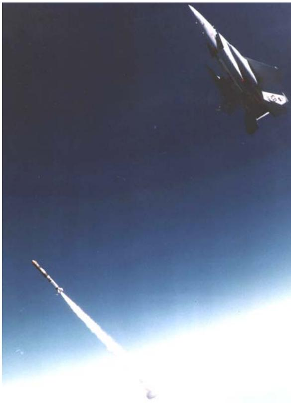
*Left: The Air-launched Antisatellite missile is released from its F-15 launching aircraft and its motor is ignited. At a certain point in its trajectory, the missile released a miniature homing vehicle which destroyed the satellite by impact. Below: A cutaway view of the ASAT's miniature homing vehicle. The rockets were mounted in an outer ring around the vehicle, and the infrared seeker assembly was in the center.*
