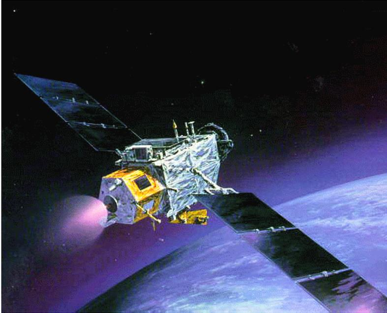
*Left: An artist's concept of the Advanced Research and Global Observation Satellite (ARGOS, STP mission P91-1) in orbit. It carried two technology demonstrations and seven high-priority experiments related to ionospheric studies, electrical systems, and electric propulsion. The experiments were provided by research agencies within the Navy, Army, and Air Force. ARGOS was launched successfully using a Delta II booster on 23 February 1999.*
