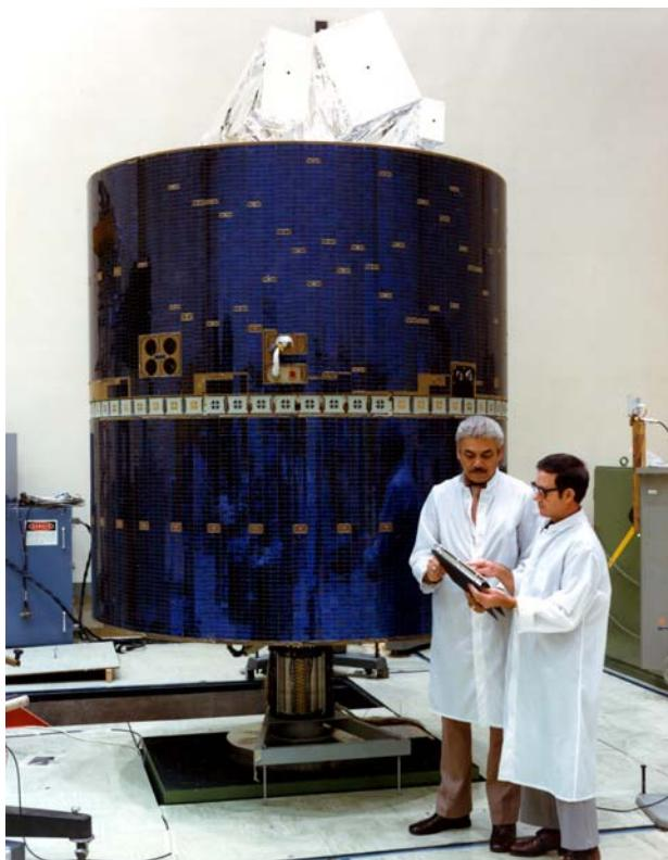
*Left: The first NATO III satellite (NATO IIIA) is prepared for testing by two technicians at Philco-Ford Corporation, the prime contractor. SAMSO launched the satellite successfully on a Delta launch vehicle from Cape Canaveral on 22 April 1976.*
