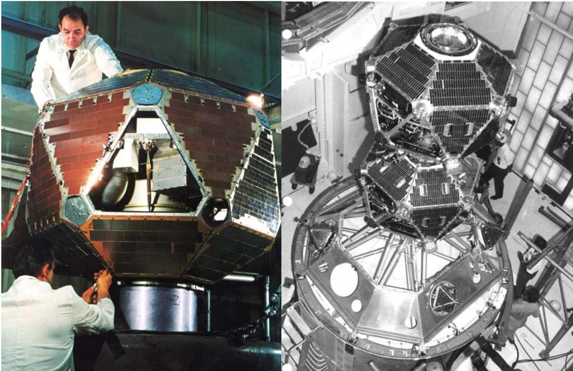
*Left: A Vela satellite in fabrication at TRW's facility. Right: A pair of Vela satellites (Vela 5A and 5B) mounted on their Titan IIIC launch vehicle before installation of the fairing. They were launched successfully on 23 May 1969.*
