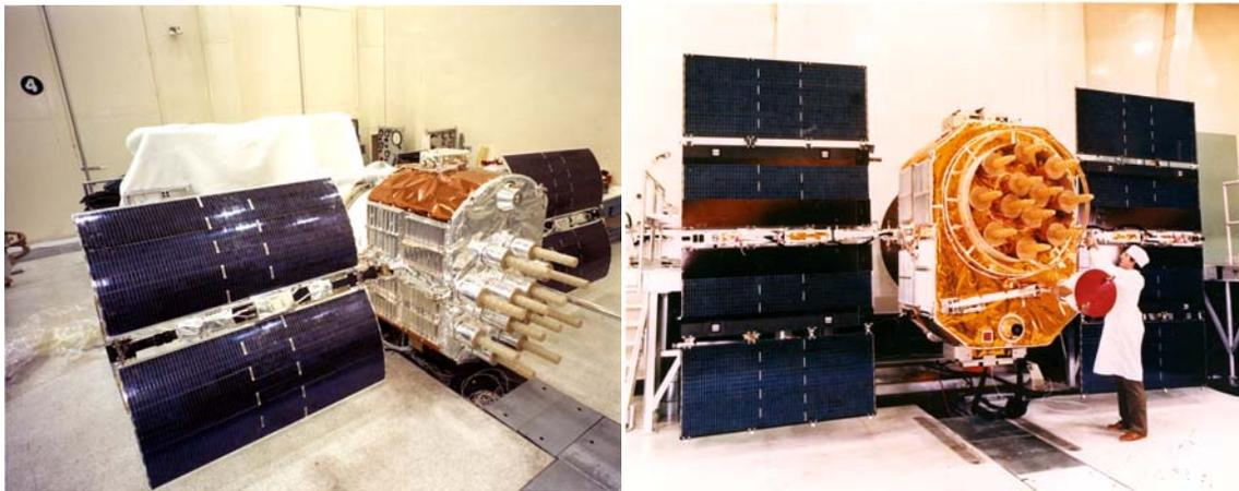
*Top: A GPS Block I satellite (left) and a GPS Block II satellite (right) undergo acceptance testing at Arnold Engineering Development Center. Bottom left: An artist's concept depicts a GPS Block IIR satellite in orbit. Bottom right: An artist's concept depicts a GPS Block IIF satellite in orbit.*
