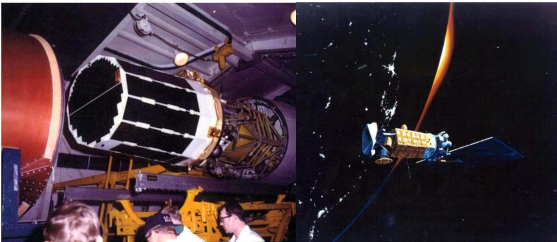
*Left: The payload fairing is being installed over a DMSP Block 5A satellite mated to a Burner II upper stage on a Thor Burner (LV-2F) launch vehicle about 1970-1971. Right: This artist's concept depicts a DMSP Block 5D-3 satellite in an early-morning orbit. The DMSP constellation consists of two operational satellites and two spares in sun-synchronous polar orbits. One of the operational satellites crosses the equator (northward) early in the morning, and the other does so at noon local time.*
