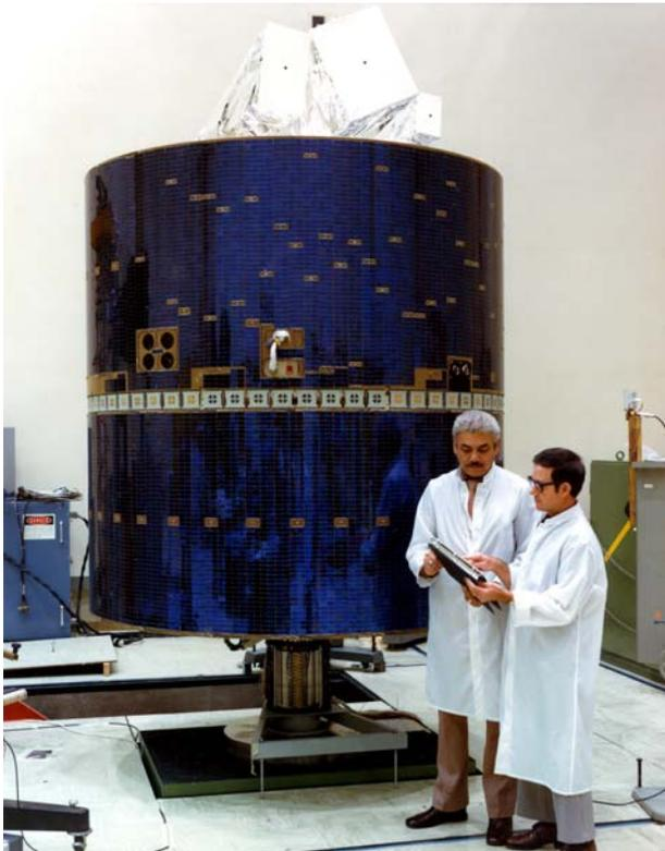
*Left: The first NATO III satellite (NATO IIIA) is prepared for testing by two technicians at Philco-Ford Corporation, the prime contractor. SAMS0 launched the satellite successfully on a Delta launch vehicle from Cape Canaveral on 22 April 1976.*
