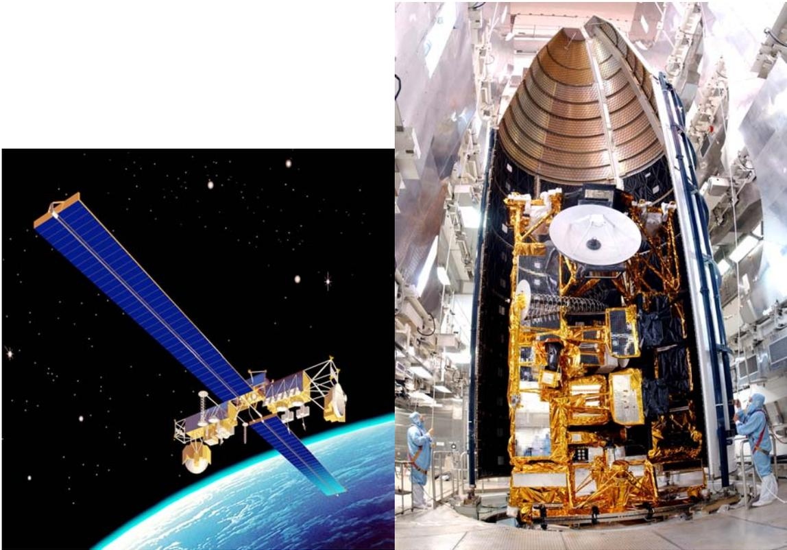
*Left: An artist's concept depicts a Milstar II satellite in orbit. Right: The fifth Milstar satellite is enclosed in the payload fairing on top of its Titan IVB launch vehicle. Its successful launch on 15 January 2002 completed the operational constellation of four Milstar satellites. (Images courtesy Lockheed Martin Missiles and Space)*
