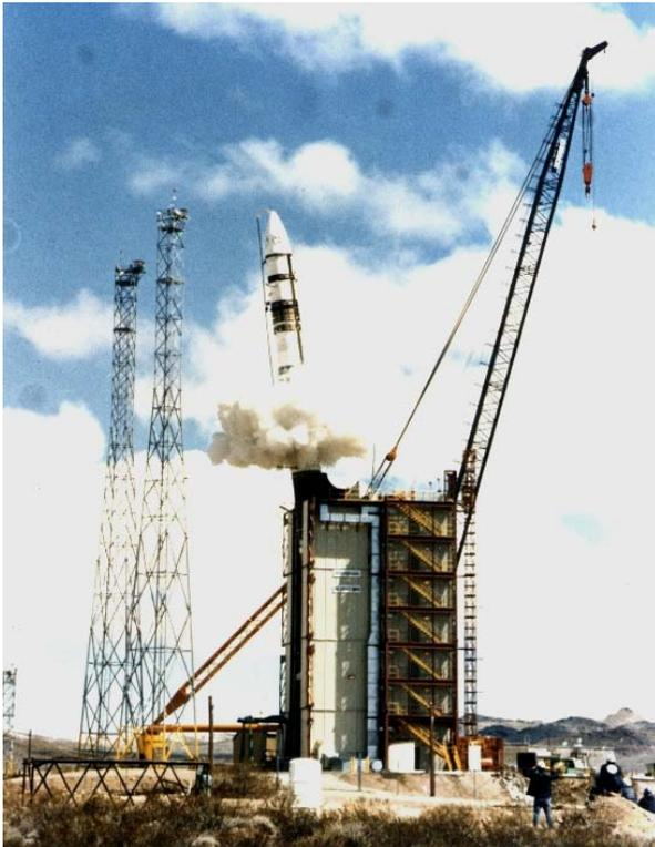
*A simulated Small ICBM being ejected from its launch canister in the Canister Assembly Launch Test Program (CALTP). Like the Peacekeeper, the Small ICBM was to be "cold launched." The missile was to be ejected from a canister, and its stage 1 motor was to be ignited after the missile was in mid-air. The CALTP program tested the launch eject system and the effects of a cold launch on stage 1 of the missile.*
