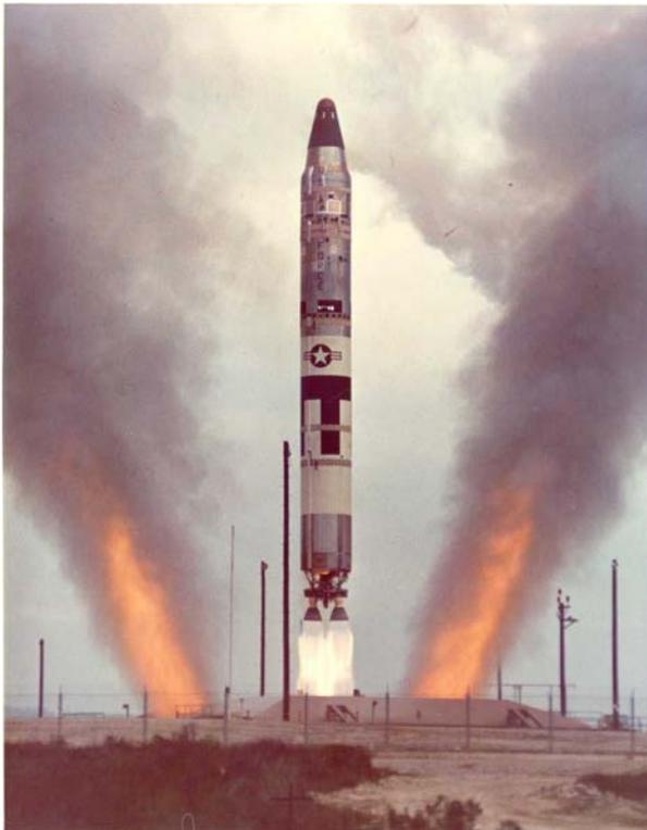
*A Titan II ICBM undergoes a test launch from an underground silo. Unlike Titan I missiles, which had to be raised to the surface before launch, the Titan II's liquid rocket engines were ignited while it was still in the silo. Therefore the silo had to be constructed with flame and exhaust ducts as shown in this photograph.*
